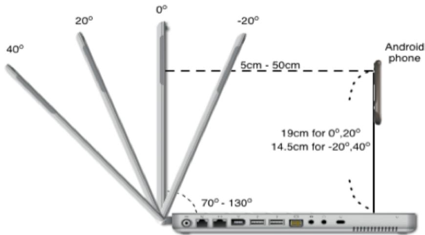
Figure 5-5: The setup of the reliability experiment.
