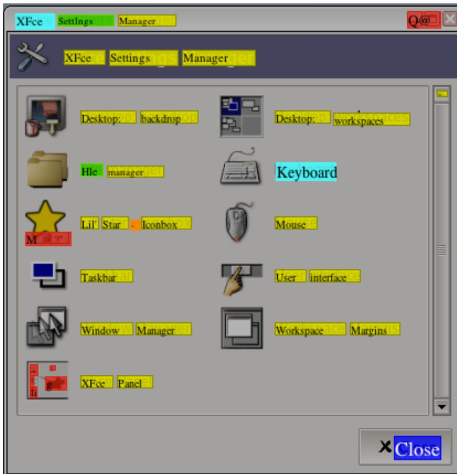
Figure 6-5: An example from the text detection experiment. Red labels are false detection, and the dark blue one is missed. All the other labels are correctly detected, but not necessarily correctly recognized.
