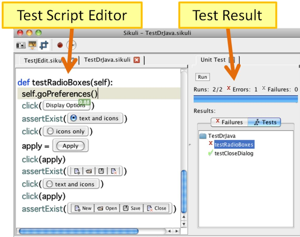
Figure 4-2: Sikuli Test interface consists of a test script editor and an information panel summarizing the test result.
