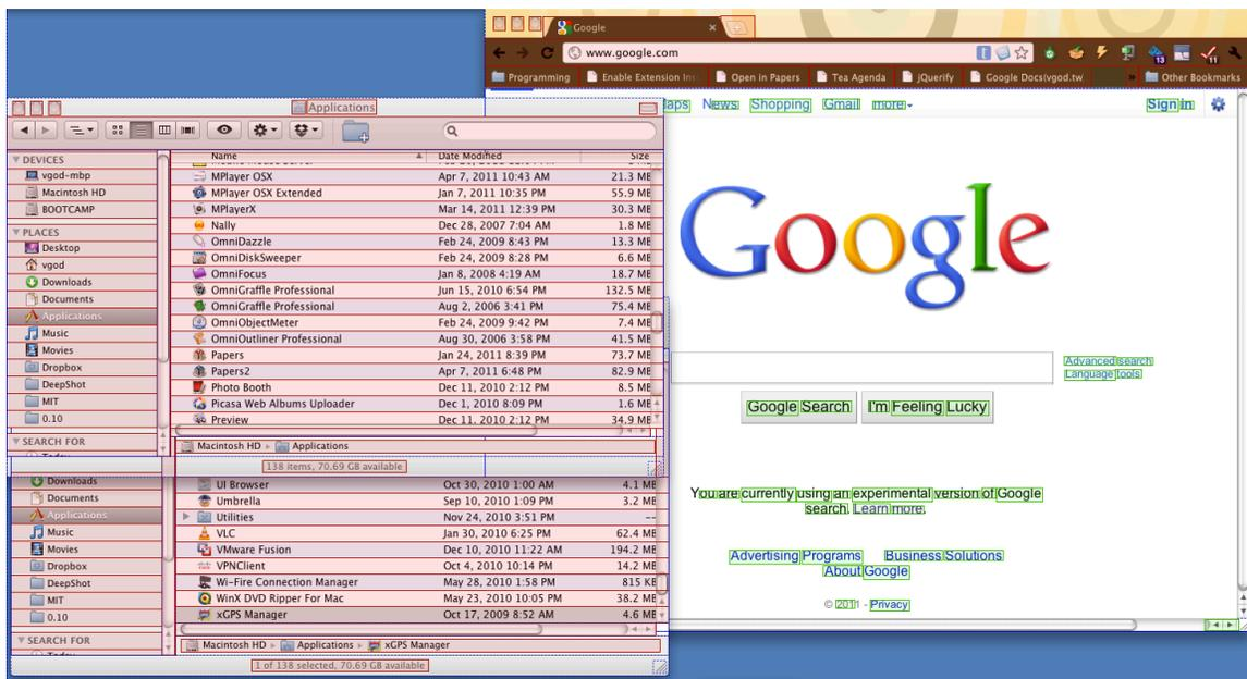
(b) PAX combines pixels and Accessibility APIs for more accurate association between the visual representation and internal structure of a GUI. It filters accessibility information for only visible objects (red boxes) and also provides role, content, location, and size of objects detected by pixel-based methods (green boxes).
