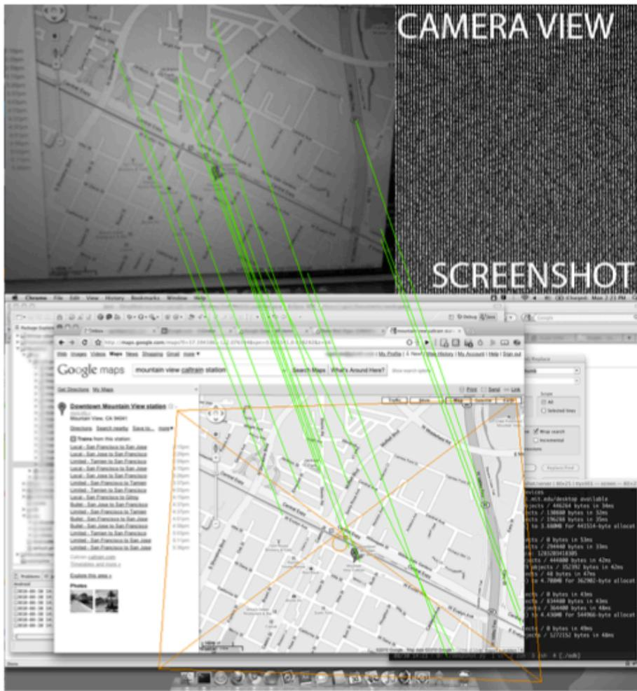
Figure 5-4: The screen matching algorithms match the picture (at the top) against the screenshot (at the bottom) and find a projective plane (the orange convex) on it.
