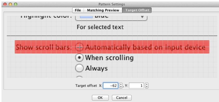
Figure 3-7: The user can adjust the click offset to the target in the Sikuli IDE.
