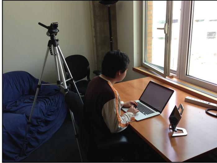
*Figure 16: Experimental Setup: a camera from behind, a computer (with webcam and driving simulation) in front, and the Android tablet on the side, as if on a dashboard*
