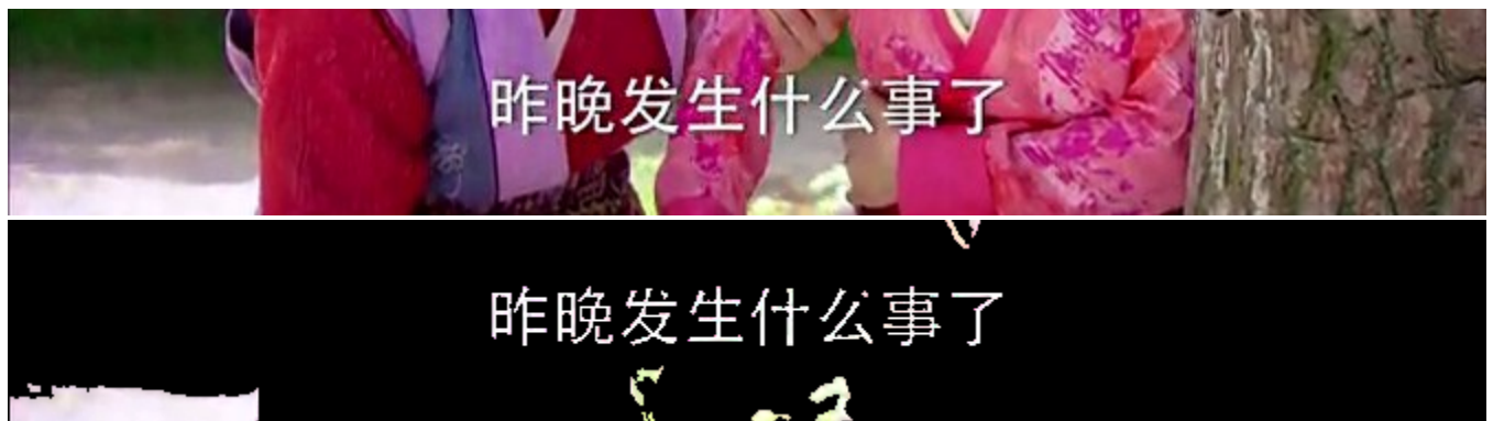
Figure 3.13: Simply extracting out the pixels which match the subtitle color results in an image with extraneous artifacts.
