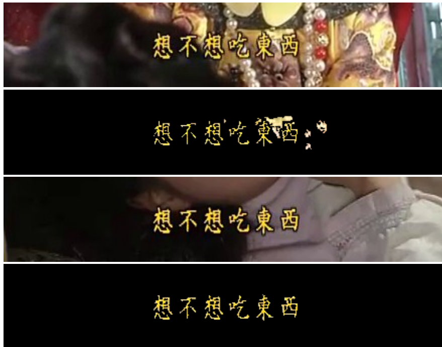
Figure 3.19: An example of why it is useful to consider multiple frames: these 2 frames both have the same text, but the second frame will have less extraneous noise after applying the noise-removal steps we described above. The pixels shared by both frames are the pixels that make up the subtitle text.
