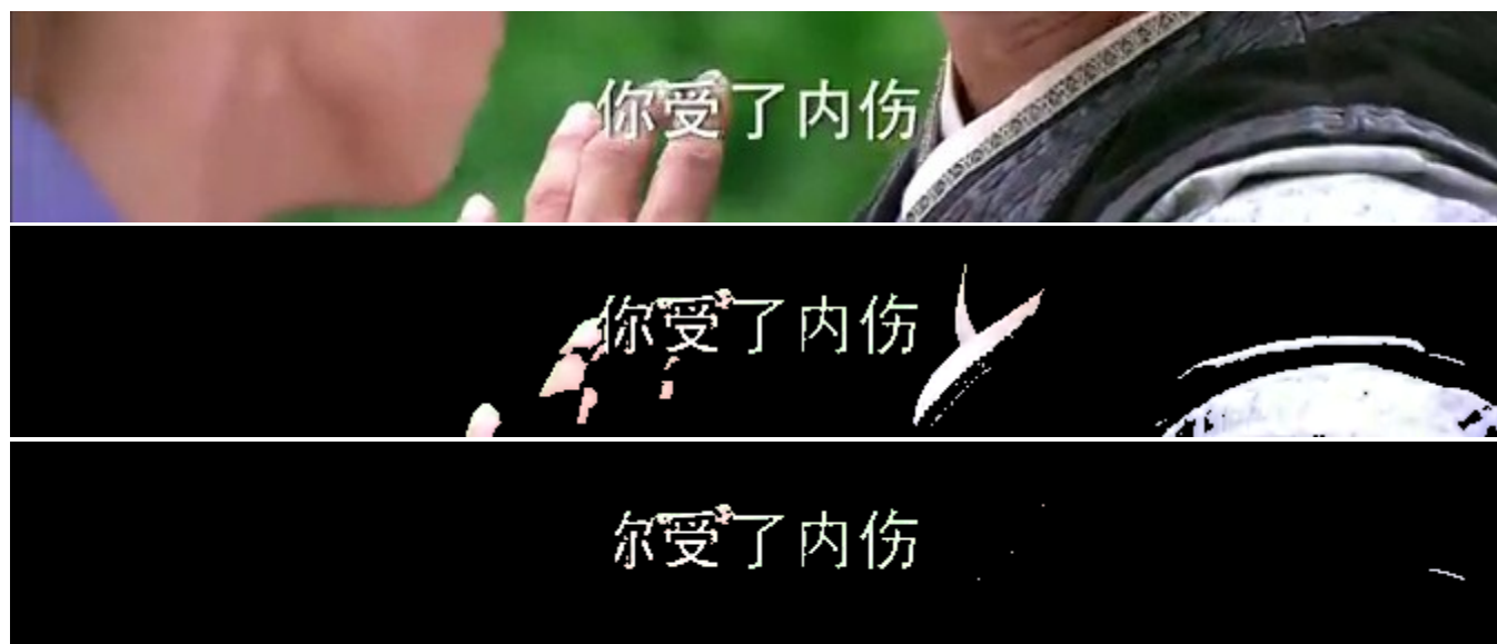
Figure 3.17 : The 亻 part of 你 was eliminated as part of the connected component-based elimination process, which will cause an OCR error later on. (尔 is a different character from 你)
